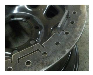
Step nine – After all of the tabs are bent upright place a weld on the outer edge of each tab as shown in the following picture.
