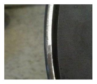
Step five - Tack weld the edge of the ring to the inner lip of the wheel, skipping around the wheel a few inches at a time.
